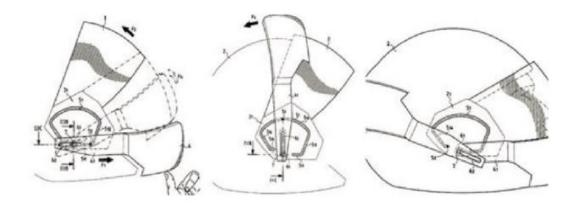
According to TECH DESIGN, figures 3A and 4A clearly showed a distinction between two different movements of "moving away" [c2] and then "raising and tilting" [c3], implying a separation between the chainguard and the shell at the beginning of the three-stage movement.
